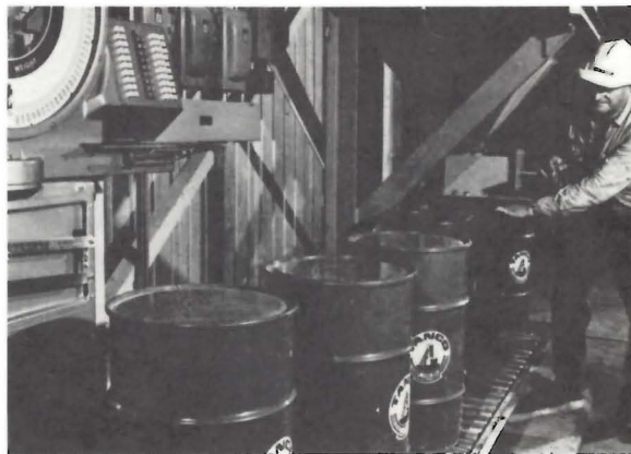
Photo 86. TANCO Mill, Packaging the Final Product for Shipment — Tantalite Concentrate, Bernic Lake (MED).
