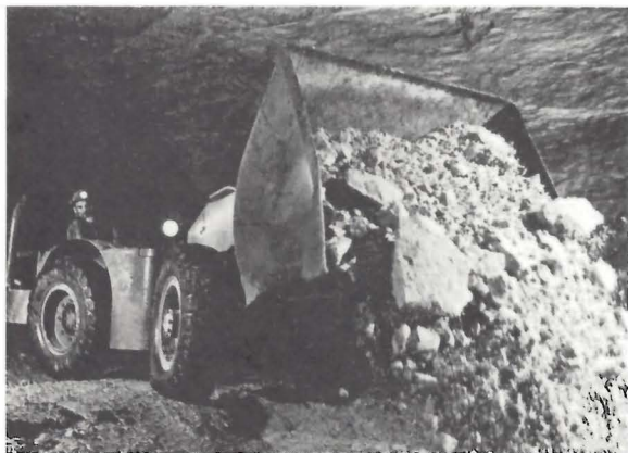
Photo 82. Dumping Muck at the Ore Pass, TANCO Mine, Bernic Lake (TANCO).
