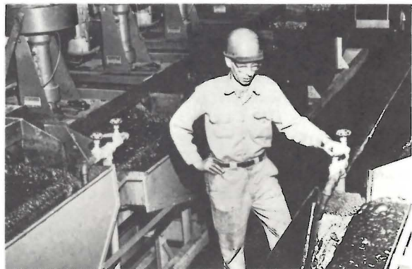
Photo 74. Thompson Concentrator, Flotation Section, Inco Metals Company. The nickel and copper sulphide particles are separated from the gangue by floating them to the surface of the pulp by aeration, agitation, and the addition of chemicals. The gangue settles to the bottom of the flotation cells (INCO).
