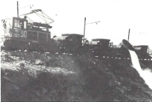
Photo 43. Slag Train, H.B.M. & S., Flin Flon. Dumping slag from the smelter (MRD).
